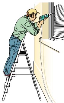
Figure 2b Correct - steps facing work activity
